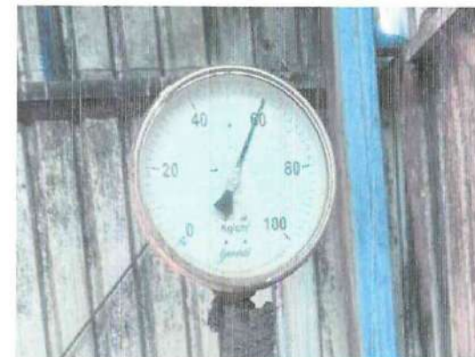
Hydrostatic test pressure 60 Barg. Holding 30 min.
