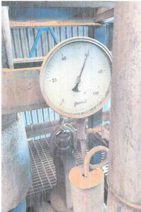
Hydrostatic test pressure 60 Barg. Holding 30 min.
