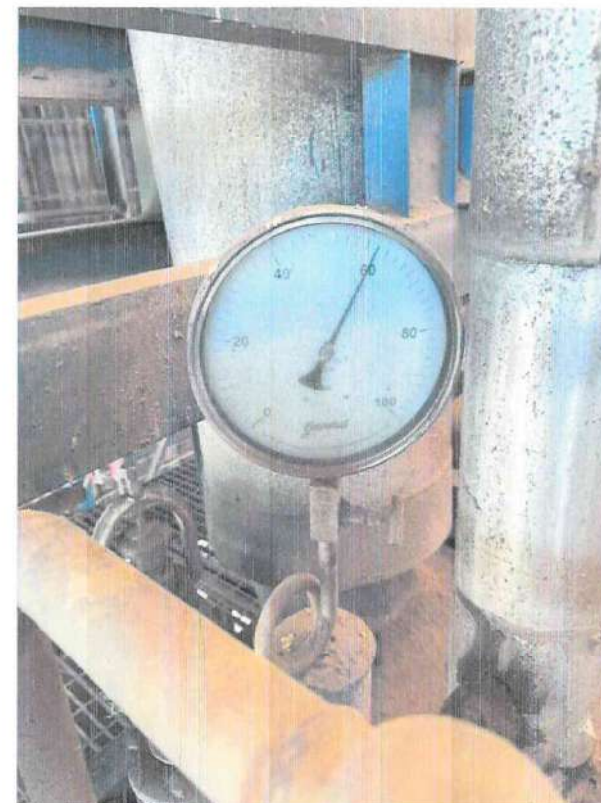
Hydrostatic test pressure 60 Barg. Holding 30 min.
